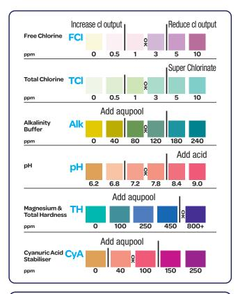
If Chlorine reading is either too high of too low, adjust output and time on your chlorinator. If consistently too low, check chlorinator cell and/or salinity level.
