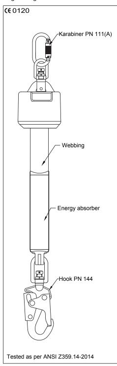
Equipped with steel Carabiner (C111) at swivel Anchorage with Load Indicator and Steel Snap Hook for attachment to the user's harness.
