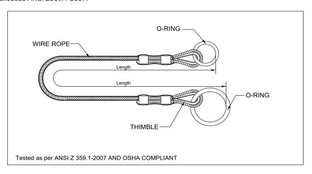
· Made of PVC coated Galvanized steel
