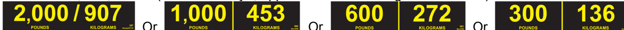
B: Label 560, 561, or 562 (both sides of jib; applied to black rectangle of label 391)
