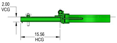
HCG = HORIZONTAL CENTER OF GRAVITY LC = LOAD CENTER LLC LOST LOAD CENTER VCG = VERTICAL CENTER OF GRAVITY
