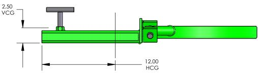
HCG = HORIZONTAL CENTER OF GRAVITY LC = LOAD CENTER LLC LOST LOAD CENTER VCG = VERTICAL CENTER OF GRAVITY
