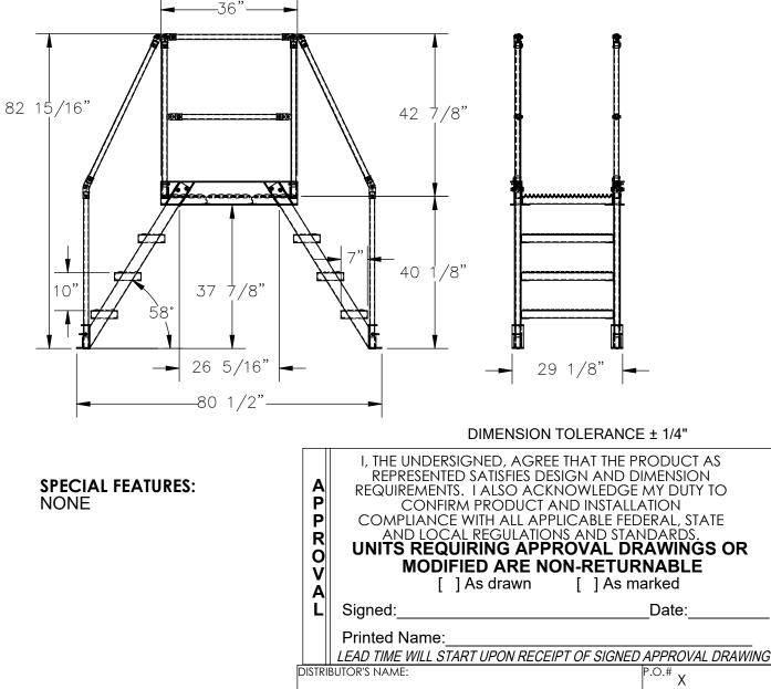
STEP HEIGHT SPACING: 10" STEP DEPTH: 7" STEP & PLATFORM WIDTH: 29 1/8" CLIMB ANGLE: 58° OVERALL CAPACITY: 500 LBS. ALUMINUM CONSTRUCTION
