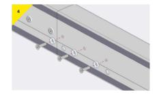
Secure the opposite side using the countersunk bolts and washers provided
