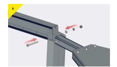
Offer one end of the beam to the rear bolt-hole on the cheek-plate (bolt 1) and insert a bolt
