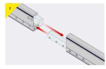
Slide the jointed beams together, ensuring the internal guide blocks are aligned correctly
