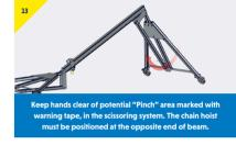
With the help of another person, scissor the beam and A-Frame into position (using the first bolt as a hinge). Be careful not to trap any fingers in this operation
