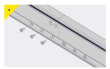
Secure the opposite side using the countersunk bolts and washers provided
