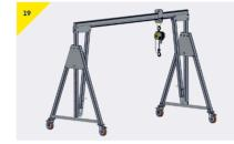
The gantry is now erect at its lowest height setting.
