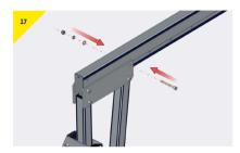
Insert and tighten the final beam bolt
