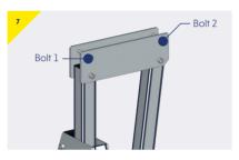
This illustration demonstrates the bolt positions (1 & 2) for the cheek plates.
