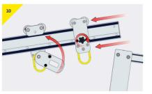
Thread the beam trolley over the other end of the beam and lock with the friction brake at approximately centre position. If using a gated trolley, lock with the friction break
