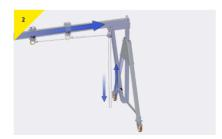
Operate the chain block to move the trolley along the beam
