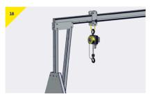
If the hoist is not already attached to the suspension point on the trolley, do so now (using stepladder if height setting requires)
