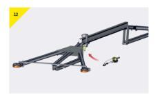
Attach the lifting device to the trolley in order to avoid having to lift and attach when gantry is fully erect.
