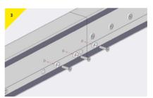
Secure one side using the countersunk bolts & washers supplied
