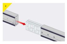
Slide the jointed beams together, ensuring the internal guide blocks are aligned correctly
