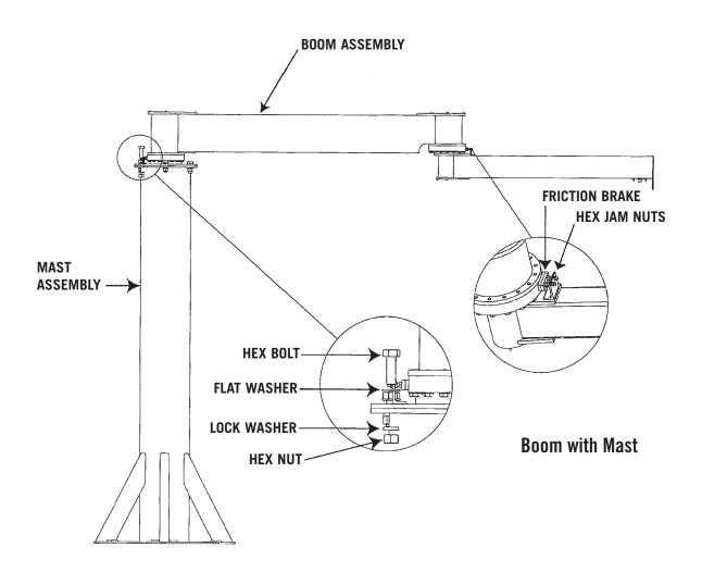
3. The Friction Brakes can now be adjusted to the desired level of resistance by adjusting the pads and locking in place with the jam nuts.
