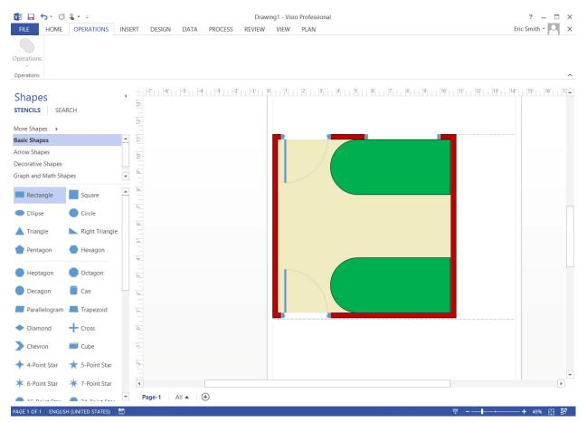
For this layout the normal minimum radius selected is to be limited to 17 in. Using this limit, care must be taken to accommodate the curvature from each of the 2 parts that have already been created. Instantiate/drag a rectangular area that connects the top and the bottom pill shapes already created. This is done by dragging a rectangle between the other rectangles along the wall. Make this
