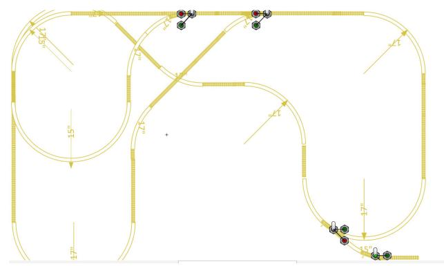
The next step is to make the track connections between sections indicated by the lamps. Don't worry that the organization of the "schematic" is incorrect as this will be corrected shortly. Draw a line for each siding that travels from the center of the lamp to the end of the siding. If space is not appropriately available, extend the line of the siding beyond the end of the track.
