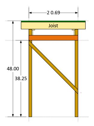
The leg "brace" should still be in the clipboard from when it was copied previously. Paste another copy of the leg and move it to where it is on the outer side of the left most leg of the riser. Select the cross brace and then the newly pasted "outside" leg and using the "Operations"-"Subtract" option, remove part of the cross brace. Repeat this process for the opposite side of the brace.
