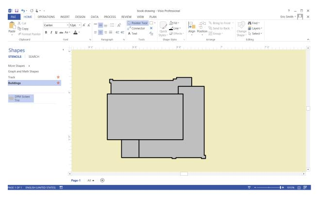
It is very advantageous at this point to "group the object" into a single entity before placing it into a Stencil. From the Home tab, select the "Pointer tool". Drag a square around the objects to put into the single shape. And either use a Control-G or from the Home tab select the Group function from the Arrange toolbox and group the objects together.
