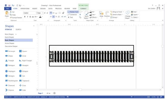
Select all of the ties and align them to the top using the "Align" menu from the "Arrange" tool option on the Home tab. To make the ties equally spaced, select one end tie first then select all of the ties and use the "Position" menu from the "Arrange" tab to "Distribute Horizontally". Lastly, fill the color of the ties with either black or a dark brown.
