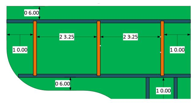
The next step is to generate the risers to support the vertical L-Girders previously put in between the horizontal L-Girders. To do this copy one of the risers already on the screen and rotate it 90°. Place a 12 in. vertical dimension object in between the two vertical L-Girders where one end meets against the horizontal L-Girder. Move the riser until it sits between the two vertical L-Girders at the 12 in. offset distance. Repeat this step to generate the other riser on the opposite end.
