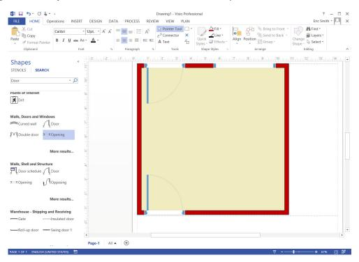
If the door or window is not on a horizontal wall, but on a vertical wall select the door with a left mouse button. A circular arrow will appear above the selected
