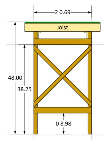
The last step with the risers, is to determine how much lumber will be required to build a riser. This can be estimated by taking a copy of the riser, placing the 2 in. x 2 in. pieces end to end, and by placing the 1 in. x 2 in. pieces end to end. (Note: one cross brace will need to be "flipped vertically" to make the ends line up. Horizontal dimension measurements can accurately show the length of each piece and the total length of the lumber necessary for a riser.
