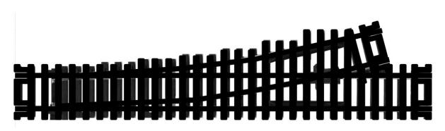
To indicate the position of the switch throw bar, draw a black rectangle from the inside of the rail to the end of the throw bar. Do not draw the switch machine in the shape because these may be hidden under the track, use an alternative switch motor, or use a manual ground throw.
