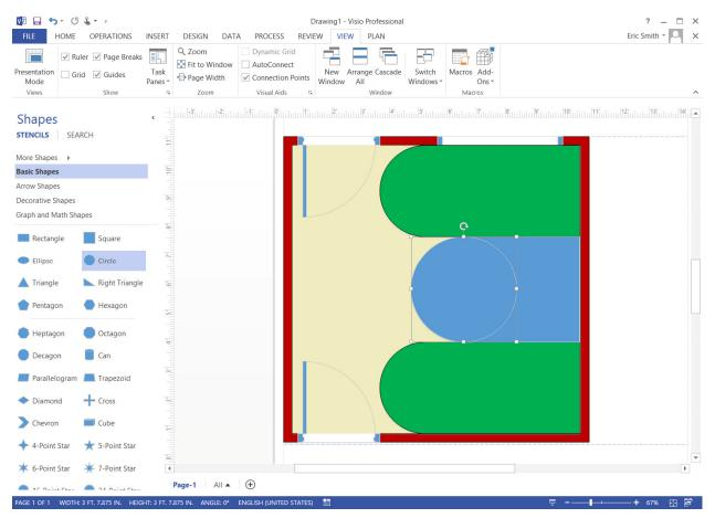
De-select the circle and select the underlying rectangle. This is because for the subtract operation, the first shape selected gets subsequent shapes subtracted from it. Hold down the "Shift" key and select the circle. Using the Operation subtract, remove the circle from the rectangle.
