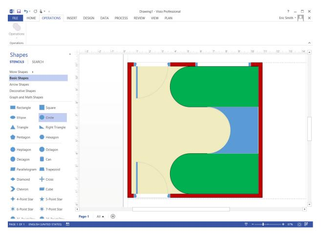
There are now 3 objects on the screen that should be one, representing the base of the layout. This is done by use of the Union command combining the 3 objects together. In the same manner as the merging of the original circle and rectangles, use the Union command to combine the base layout objects. Once again order is important to keep the color of the first select object.
