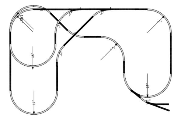
In the tutorial diagram, there are 6 switch machines, two sidings and one loop that will need isolation and be implemented as a reversing loop. The schematic of the drawing layout can be reduced to showing the major areas as follows:
