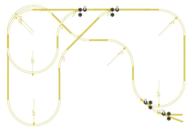
Before starting the next step of drawing the lines between the lamps and toggles, verify that the snap features are all turned on. On the View tabs under the visual aids additional capabilities in the "Snap & Glue" dialog make sure all of the snap options are selected. This allows a line to be drawn from one object to another such that when the object is moved, the line will move with the object.
