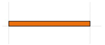
Drag a Dimensioning – vertical object to the screen and move it around until the top of the measurement object meets with the guideline. A small green square will appear indicating it is okay to snap to the guideline. On the opposite end of the measurement object stretch it until it is 38 1/4 in. in height. Drag a guideline from the top ruler until it meets up with the bottom of the measurement object.
