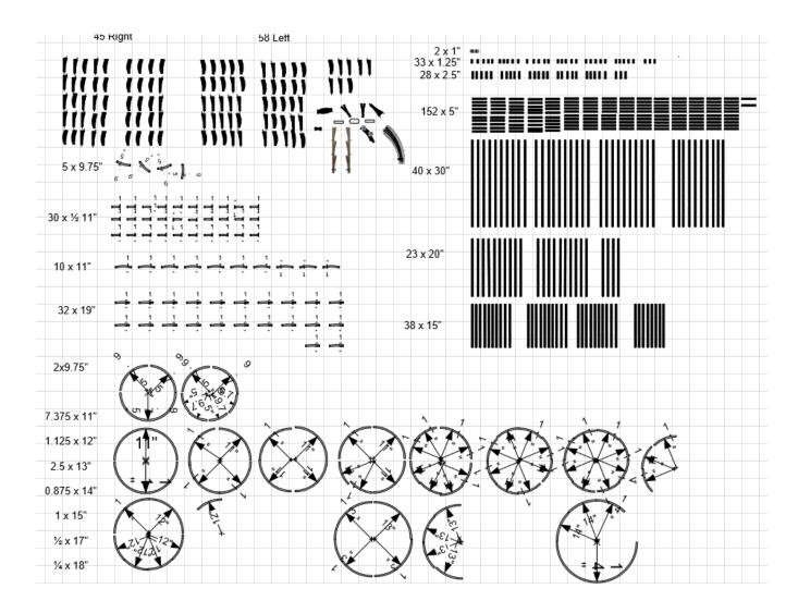
A benefit of this organization is that with a count of the individual components, even the amount of cork required for the track can be calculated by summing up the amount of track in the inventory. Curve radius length (circumference) is calculated by using the formula:
