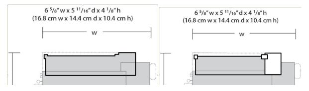
To draw the right side, draw 2 rectangles representing the depth and width of the right side of the picture and the longer bottom side picture. To get the correct shape union these two shapes together.
