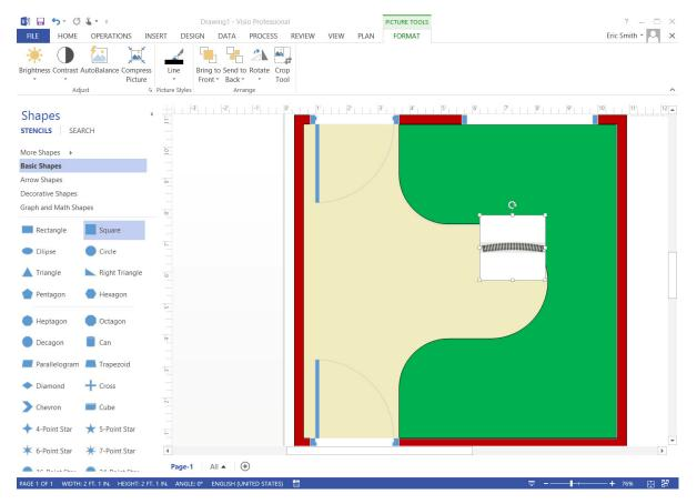
From this image it can be seen that the picture was inserted of a 24 in. Radius track picture that is 2 ft. 1 in. in length and height. The radius of the curve is measured from the center of the curve which means this piece of track in the picture is over twice the size necessary to represent the actual track.
