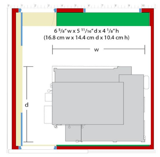
With the dimensions of the kit known, it is possible to shrink the image proportionally to the correct size by using the small white selection boxes on the corners of the picture. However, to get it to the correct size it is recommended to draw a rectangle that exactly matches one of the dimension on top of the picture. Use the width dimension on the picture for this effort.
