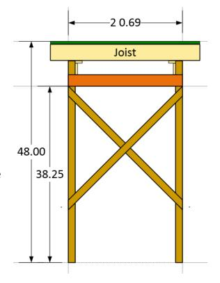
To complete the riser a horizontal component should be added to guarantee that the riser will not move. Use the top piece of the riser (this is the one copied from the other page) for the horizontal rectangle/stabilizer. If more stability is required a second horizontal stabilizer can be added at the bottom of the cross braces.
