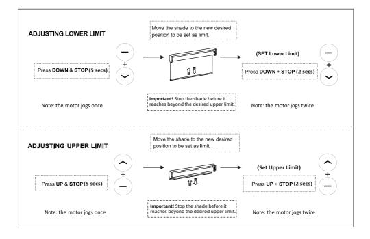
**Tips:** If you hold the UP/DOWN button for more than 3 seconds, the shade will enter running mode. As the shade approaches the desired limit, press the STOP button and then fine-tune the limit.
