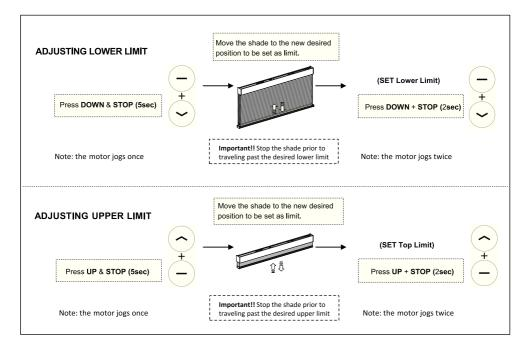
!!WARNING!! - Move shade in short increments by pressing the UP/DOWN button in 1 second intervals (pressing the UP/DOWN button for more than 3 seconds may send the shade past desired upper/lower limit and may result in damage to the product). Once you have reached the desired upper/lower limit, you can adjust the limit with either the UP and DOWN buttons. (remember to adjust in short increments!)
