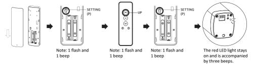
Note: Please ensure that the displayed channel on the remote corresponds to the shade you intend to adjust. When pressing the 'up' button, the 5-channel remote should not display all 5 indicators lit up, and the 15-channel remote should not show as 0.
