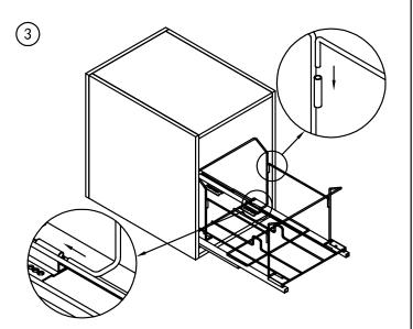
Insert 2pcs of support bars into the bottom tube according to the arrow direction shown in the figure, and then insert 2pcs of U-shaped bars into the tube according to the arrow direction shown in the figure to complete the third step.
