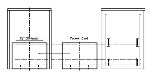
Align the arrow direction of the paper card with the edge of the cabinet, place the center line of the paper card on that of the cabinet, and use a 2.5-mm drilling bit to drill holes on the baseboard of the cabinet. Align the left and right guide rails with the holes shown in the figure, and secure the first
