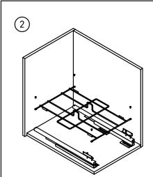
As shown in the figure, fix the door panel connector 1 and slide rail with 2pcs M4x8mm screws. Then, fix the baseboard with 4pcs M5x8mm screws to complete the second step.
