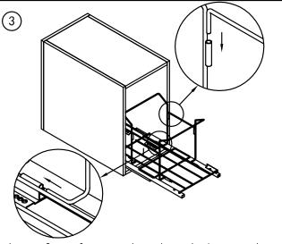
Insert 2pcs of support bars into the bottom tube according to the arrow direction shown in the figure, and then insert 2pcs of U-shaped bars into the tube according to the arrow direction shown in the figure to complete the third step.
