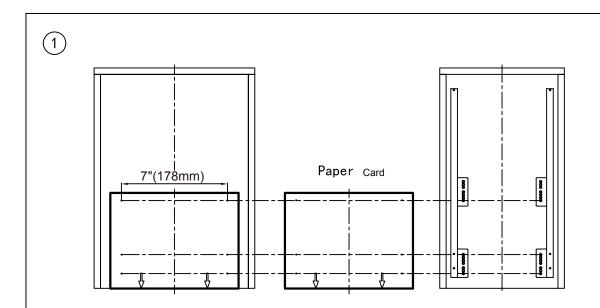
Align the arrow direction of the paper card with the edge of the cabinet, place the center line of the paper card on that of the cabinet, and use a 2.5-mm drilling bit to drill holes on the baseboard of the cabinet Align the left and right slide rails with the holes shown in the figure, and secure the first step with six ST4x14mm self-tapping screws.
