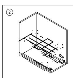
As shown in the figure, fix the door panel connector 1 and slide rail with 2pcs M4x8mm screws. Then, fix the baseboard with 4pcs M5x8mm screws to complete the second step.
