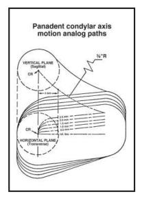
A schematic of the Motion Analogs show the variations in the curved Bennett pathways, in the functional range of 3mm from centric relation. The Motion Analogs have been created with the 3/4 inch radius superior wall and 6° orbiting pathways.
