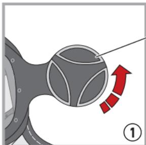
To remove the visor, release the side cover **A** by turning it anti-clockwise **1**.
