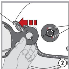
To install the visor, starting from one side of the helmet, align the coupling holes **D** with the slider pins **C** **3**.
