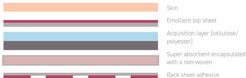
..... FIGURE 4: EXPOSURE RISK OF DIFFERENT LAYERS OF DISPOSABLE PADS
