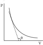
The variation of P with V at constant heat content is represented by an Adiabatic curve.
