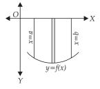
(iv) It may also happen that some portion of the curve is above *x*-axis and some portion is below *x*-axis as shown in the figure. Let  $A_1$  be the area below *x*-axis and  $A_2$  be the area above the *x*-axis. Therefore, area bounded by the curve y = f(x), *x*-axis and the ordinates x = a and x = b is given by
