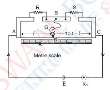
Potentiometer Setup for Comparison of emf's of two cells :
