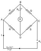
The Wheatstone bridge is balanced when there is no current flow through the galvanometer. It means potential at B is equal to that at D. In such a case
