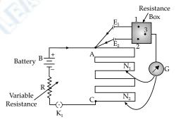
Potentiometer Setup for Evaluation of Internal Resistance of a cell:
