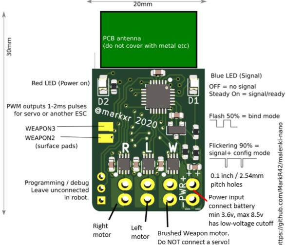
Brushed motor outputs: full battery voltage, 1.8A max current per channel
