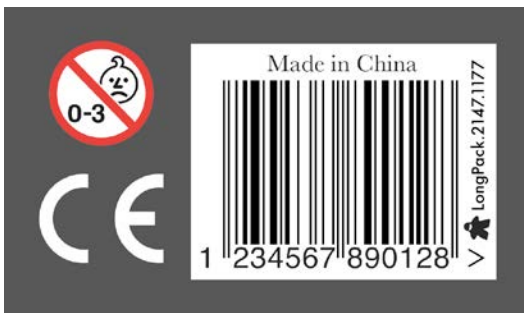
Example of Choke warning, CE marking and LongPack games lot number placement.
