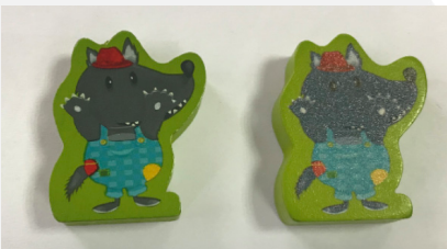
5.7.6 • Example of the UV printing color issue ( Left: Heat Transfer printing • Right: UV Print )
