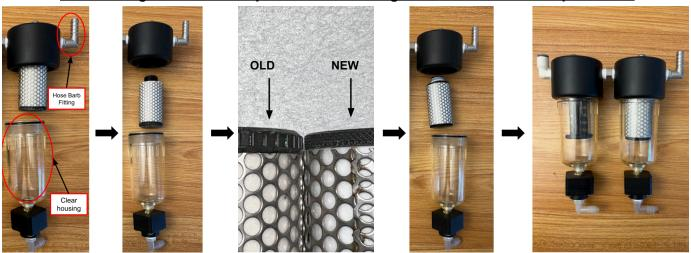
15. Remove the clear housing from the black filter body with the metal 90° hose barb fitting
