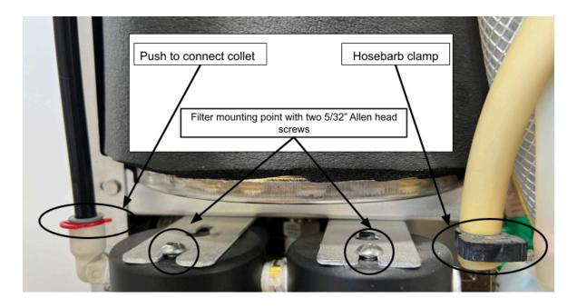
24. With the filter mounted we can attach the drain tubing.
