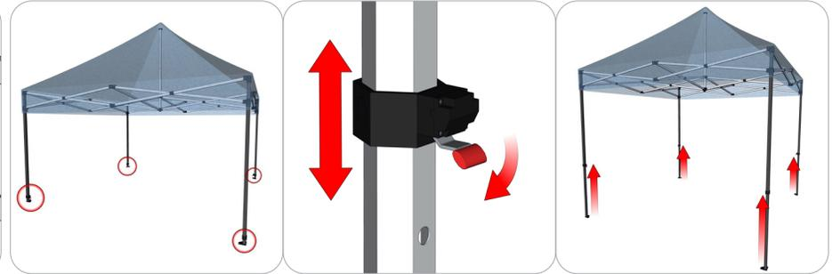
At two adjacent corners of the tent, slide the inner legs up until the snap button locks into the hole of the outer leg. Repeat with the remaining two legs. Minimum of two people recommended.
