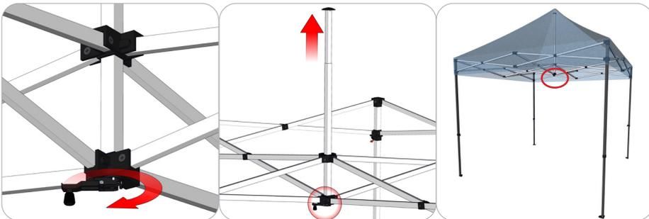
The frame will have one canopy tensioner at the center of the underside. Carefully turn the lever clockwise to create tension on the canopy. This will raise the canopy and eliminate wrinkles.
