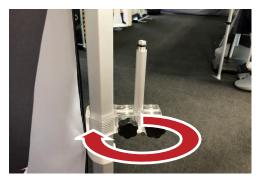
**Step 3.** Unscrew the pole pin wing nut, slide the pin through the accessory piece hole, and lock in place with the wing nut.
