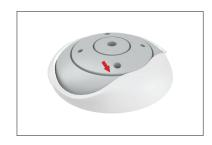
**Step 7:** Insert display frame into base by pushing post into hole.
