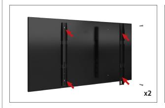
**Step 4:** Insert base plate pole through front of graphic.
