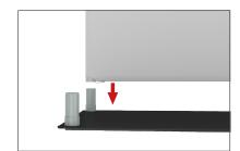
SHELVING & ACCESSORIES: (OPTIONAL) To add shelves or accessories to frame, position and level part on frame before tightening clamps down with hex tool.
