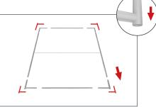
**Step 6:** Push banner stand frame onto back posts of flat base or optional feet. Press evenly on both sides to make easier for the frame to go on.
