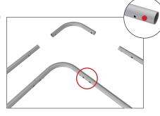
**Step 6:** Zip the edge of graphic beyond the center point as shown to hold the center pole in place. Zip the remaining side and bottom to
