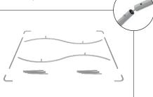
**Step 2:** Connect all corner sections to curved and straight sections of the frame by matching shape symbols on pipes.
