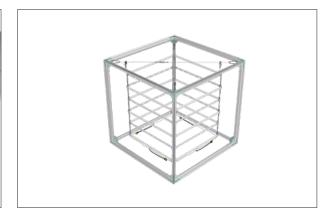
**Step 8:** Fit PVC inner boards onto the top of frame with wedge side face down. Position and align boards until they are all fitted down into the frame.
