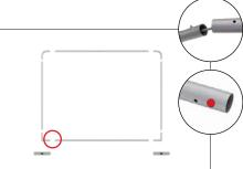
Step 4: Unzip print and lay image face down. Slide print onto the frame like a pillow case.
