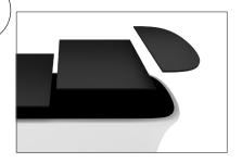
**Step 4:** Join counter top panels together front and back with black push-on clamps.
