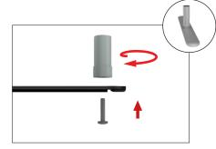
**Step 5:** Push banner stand frame onto posts of flat base or optional feet. Press evenly on both sides to make easier for the frame to go on.
