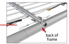
Step 7: Find cable ends and pull through grommet holes. Connect each power cable to a power supply. WARNING! Only connect one light array to each power supply.
