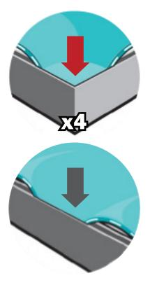
Fit graphic into corners, then "tap" into rest of frame channel.
