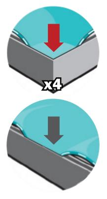
Fit graphic into corners, then "tap" into rest of frame channel.
