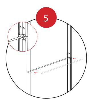
Fit the Channel Bar ◆ into place on the Side Extrusions.
