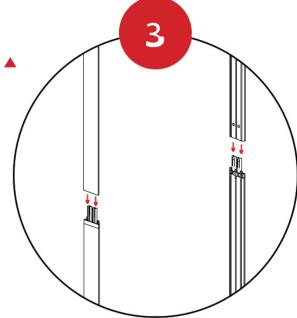
Fit the Top Extrusions together.
