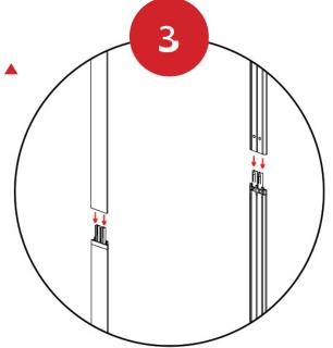
Fit the Top Extrusion onto the Side Extrusion Top connectors.
