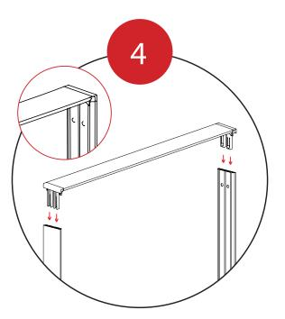
Fit the Channel Bar ◆ into place on the Side Extrusions.
