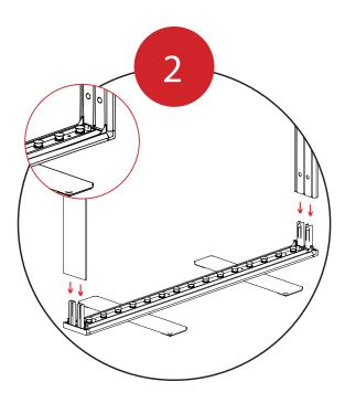
Fit the Side Extrusion Tops A onto the Side Extrusion Bottom connectors.
