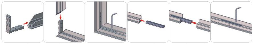
First, insert the corner connector into the extrusion. Then, slide the next extrusion onto the same corner connector. Finally, hold the corner components together and use the provided Allen Key to lock the corner connector in place.
