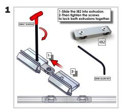
Using the 5mm Allen-T attach your PMFC2s together with your IB2s like the instructions here.
