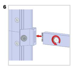
Using the 5mm Allen-T attach your supporting PH1 extrusions to your brackets.
