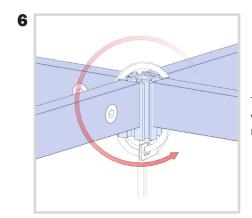
To attach lights to the tower simply wrap the cords around the joints in the middle of the frame.
