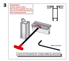
Using the 5mm Allen-T attach your PHFC2s to your PMFC2 verticals made in the previous step.
