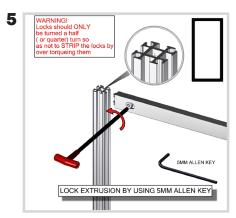
Using the 5mm Allen-T attach your supporting PH1 extrusions to the small PX extrusions.
