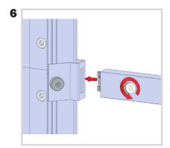
Using the 5mm Allen-T attach your supporting PH1 extrusions to your brackets.
