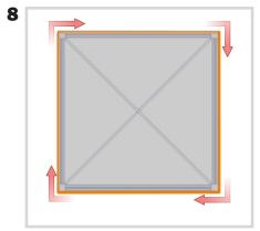
Your opaque liner will attach to the top of your tower with hook and loop fastener on the liner and on the top of the extrusion.
