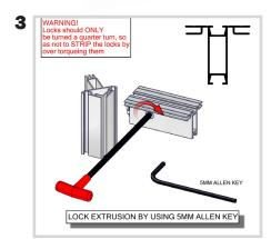
Using the 5mm Allen-T attach your PHFC2s to your PMFC2 verticals made in the previous step.
