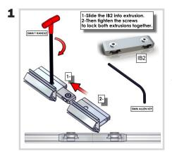
Using the 5mm Allen-T attach your PMFC2s together with your IB2s like the instructions here.
