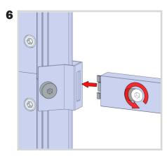
Using the 5mm Allen-T attach your supporting PH1 extrusions to your brackets.
