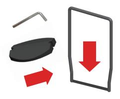
Note: You may need to pull the SWING-SIGN-FRAME up while pushing down on the SWING-SIGN-BASE to ensure a secure fit.
