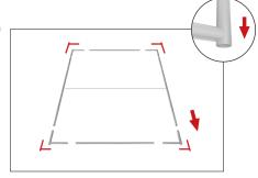
Step 6: Push banner stand frame onto back posts of flat base or optional feet. Press evenly on both sides to make easier for the frame to go on.
