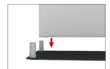
(OPTIONAL) To add shelves or accessories to frame, position and level part on frame before tightening clamps down with hex tool.
