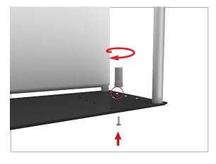
LIGHTS: (OPTIONAL) Position as desired and tighten knob to hold in place. WARNING! Over tightening may cause damage to fabric image.
